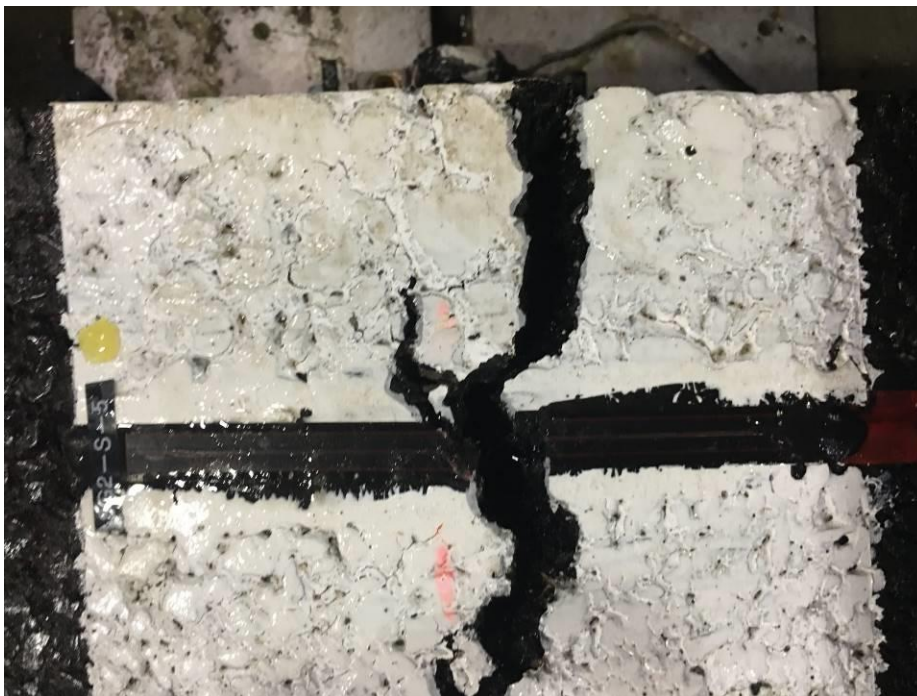
Fig 7 South section surface crack reached the inner vertical edge
