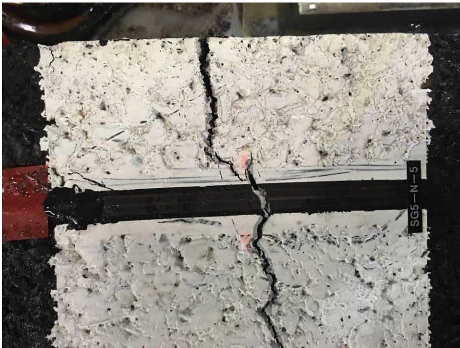
Fig 3 Surface crack on North Section reached outer edge
