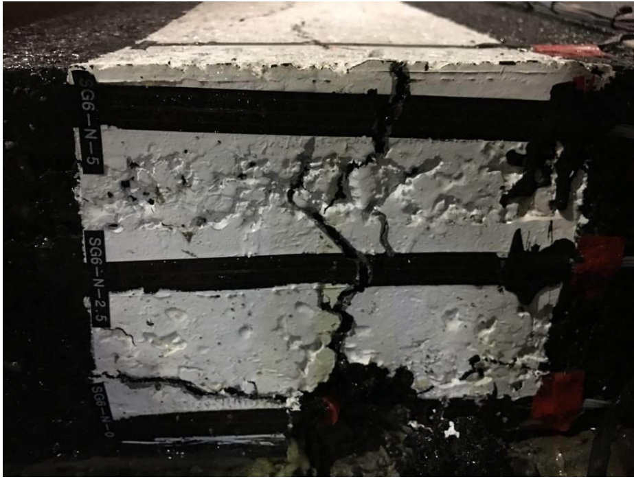
Fig 2 Bottom-up crack at north section outer edge reached top surface
